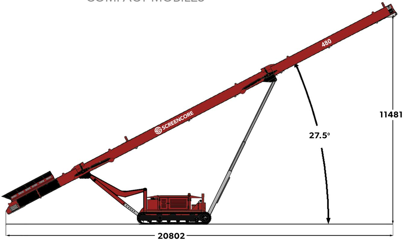
**The Screencore 480 is a 24m tracked stacker with twin drive and 1200mm belt for heavy-duty applications.**
