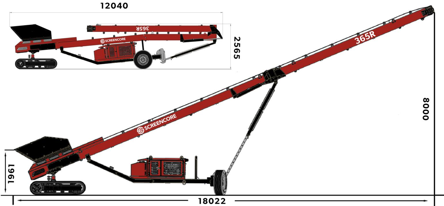
**The Screencore 365R is a heavy-duty 19m tracked radial stockpiler giving the operator ultimate flexibility with material movement and placement.**
